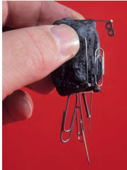
Not all magnets are man-made; certain rocks (for example, this piece of magnetite) are naturally magnetic.
