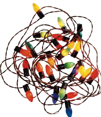
▲ These coloured lights are connected in series – if you take one out they all go out.
