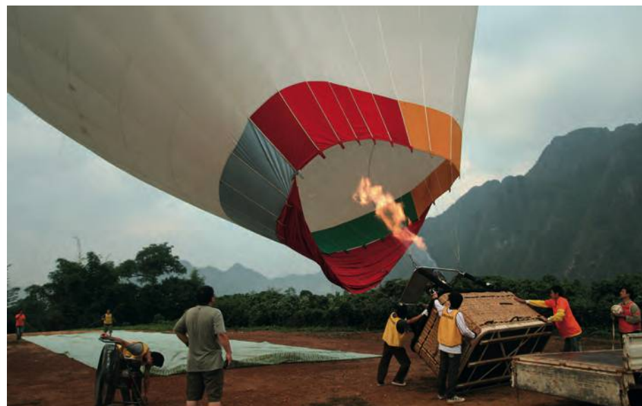
Figure 8.3 Underneath the balloon is a flame which heats the air in the balloon and this drives the engine.
