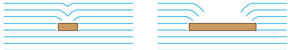
Figure 5.54 Diffraction around obstacles.
